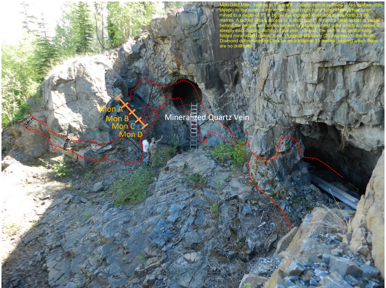
Photo 2. Crown Pillar of A Zone showing mineralized Quartz Vein and Location of Verification Chip Sampling (labeled Mon A to D respectively).
