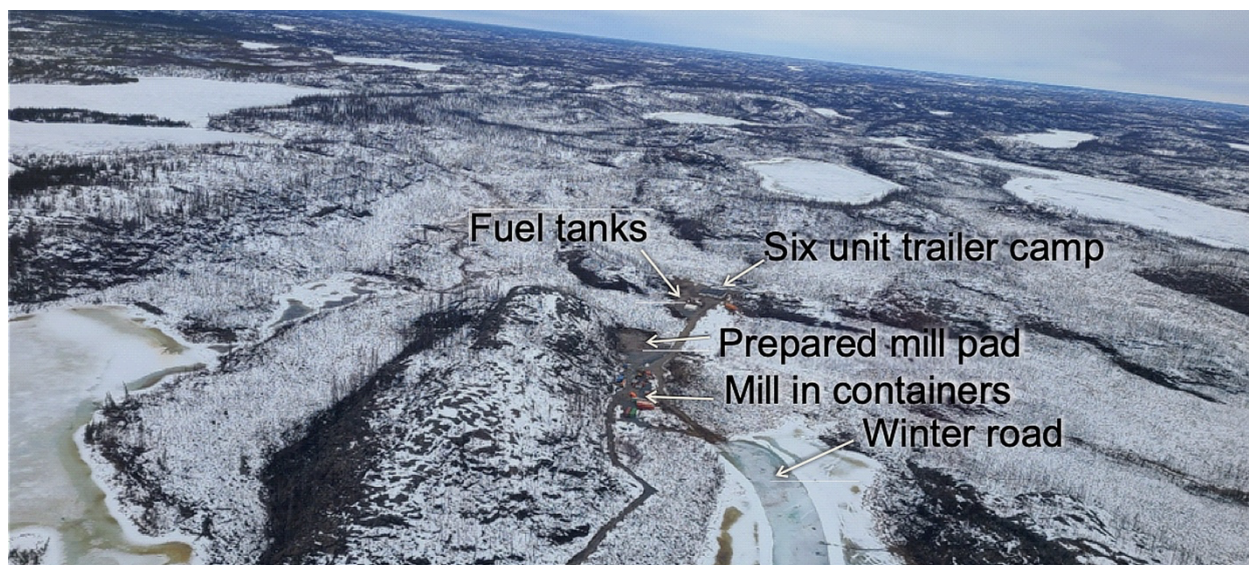
Photo 1. Northeast view of the Mon Gold Mine site May 6, 2026 showing light snow on the ground and the still frozen lakes. The camp is in place mid-photo and the containers containing the mill are located next to the mine shops, compressors and generators, south of the blasted mill pad.
